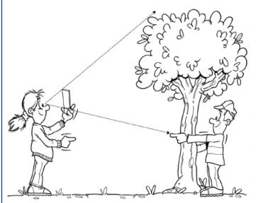
Ratio stick. Cut a strip of card so that it is exactly 30cm long and approximately 3-4 cm wide. Exactly 3cm from the bottom draw a line or arrow across the whole width. You are now ready to calculate tree heights.
